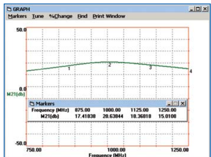
Figure 6: Amplifier Frequency Response (Initial Synthesized Circuit)
