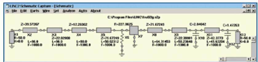
Figure 5: LINC2 Synthesized Amplifier Schematic
