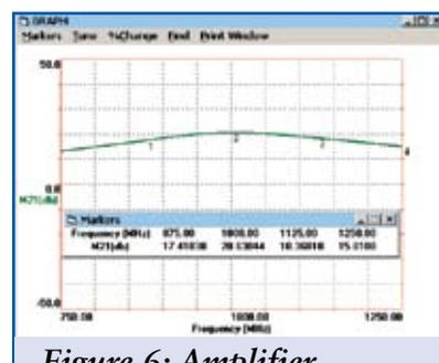
Figure 6: Amplifier Frequency Response (Initial Synthesized Circuit)
