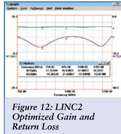
Figure 12: LINC2 Optimized Gain and Return Loss
