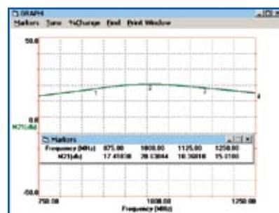
Figure 6: Amplifier Frequency Response (Initial Synthesized Circuit)
