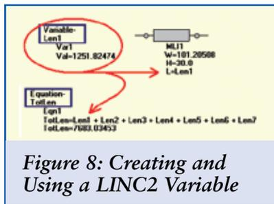
Figure 8: Creating and Using a LINC2 Variable
