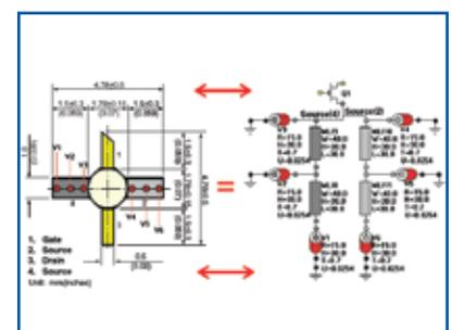
Figure 7: FET Source Grounding with Multiple Ground Vias
